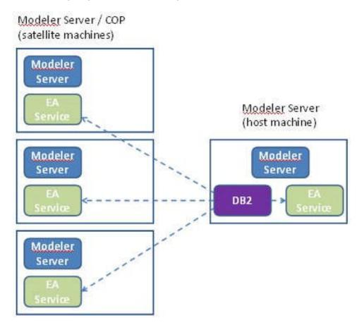
Figure 2 – Modeler Server – Configuration of COP Cluster Machines
