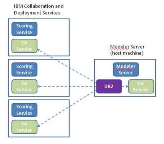
Figure 1 – C&DS – Configuration of Cluster Machines
